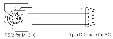
Figure 6.21: Interface connection for data transfer over PC COM port
