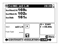
Figure 5.39: Example of 2  $\Omega$  line/loop measurement results
