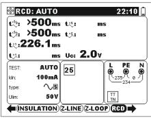
t∯: >500ms t∄: t:::226.1ms (t;:,:226.1ms ∪c: 2.0v **А**∪ТО 26 TEST: ldn: 100mA ^\s type: Ulim: 50 V (INSULATION)(Z-LINE)(Z-LOOP)(RCD) Step 3 Step 4 RCD: AUTO
