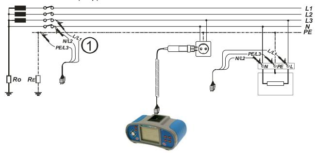
Figure G.6: Connection for reference (1) and socket measurements
