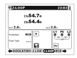
Figure E.4: Fault loop impedance
