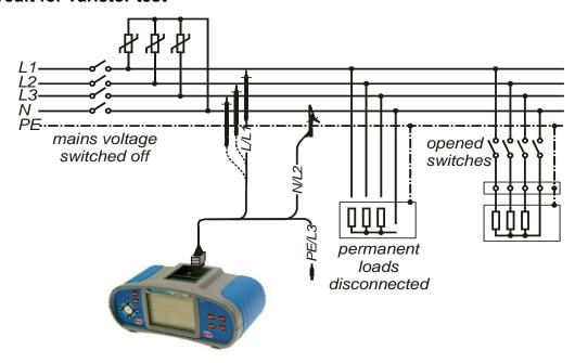
Figure 5.47: Connection of universal test cable for varistor test
