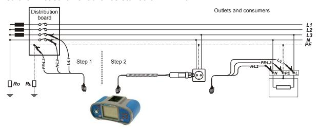
Figure F.1: Two step procedure for PE wiring resistance measurement – connection of plug commander and universal test cable
