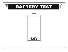
Figure 2.1: Discharged battery indication
