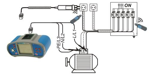
Figure 5.43: Tracing wires under walls and in cabinets
