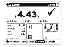
Figure 5.20: Examples of loop impedance measurement result
