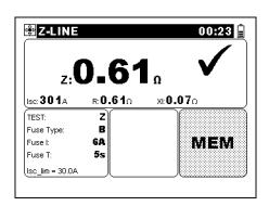
Figure 6.9: Stored single test example
