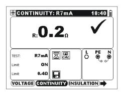
Figure 5.9: Example of 7 mA resistance measurement
