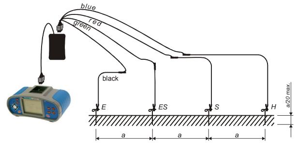
Figure 5.35: Specific earth resistance measurement with  $\rho$ -adapter
