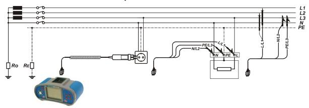
Figure 5.23: Phase-neutral or phase-phase line impedance measurement – connection of plug commander and universal test cable
