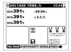
Figure 5.30: Examples of voltage measurement in three-phase system
