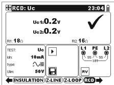
Figure E.3: RCD Uc test
