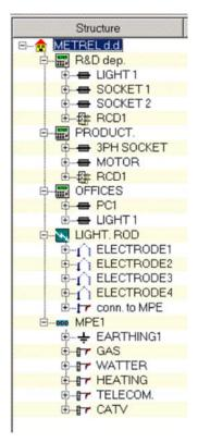
Figure 6.2: Installation structure example as presented on PC
