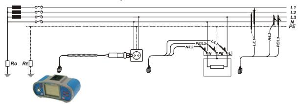
Figure G.12: Phase-neutral or phase-phase line resistance measurement – connection of plug commander and universal test cable
