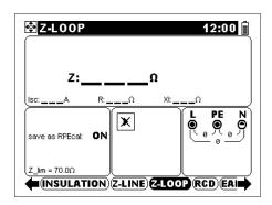
Figure G.8: Fault loop impedance
