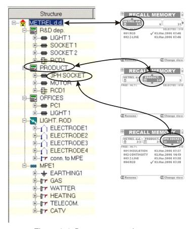
Figure 6.4: Data structure elements
