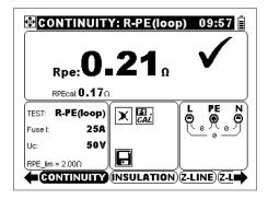
Figure G.7: Example of continuity R-PE(loop) result
