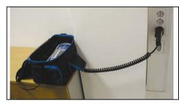
The instrument can be used even when placed in soft carrying bag – test cable connected to the instrument through the front aperture.
