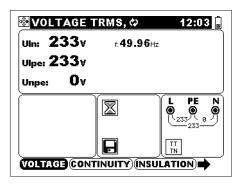
Figure 5.27: Voltage in single phase system
