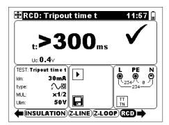
Figure 5.15: Example of trip-out time measurement results
