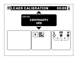
Figure 5.10: Test leads resistance compensation menu
