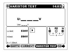
Figure 5.46: Varistor test menu
