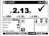
Figure F.7: Examples of loop impedance measurement results
