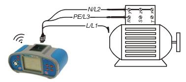
Figure 5.8: Universal test cable application
