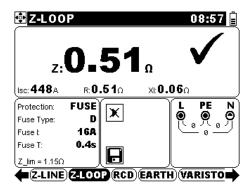
Figure F.1: Examples of loop impedance measurement result
