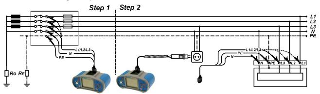
Figure 5.25: Phase-neutral or phase-phase voltage drop measurement – connection of plug commander and 3-wire test lead
