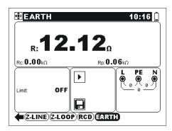
Figure 5.34: Example of resistance to earth measurement result
