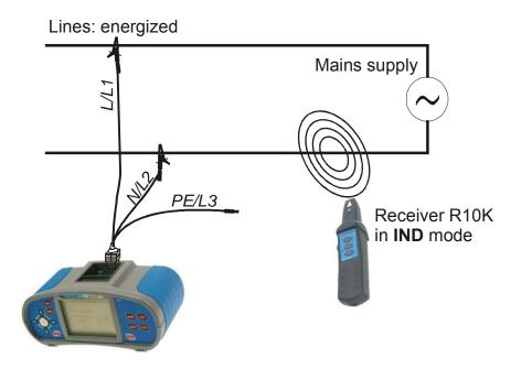
Figure C.3: The EurotestAT as a signal source for tracing lines
