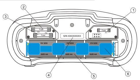
Figure 3.4: Battery and fuse compartmentLegend:
