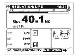
Figure 5.4: Examples of insulation resistance measurement results
