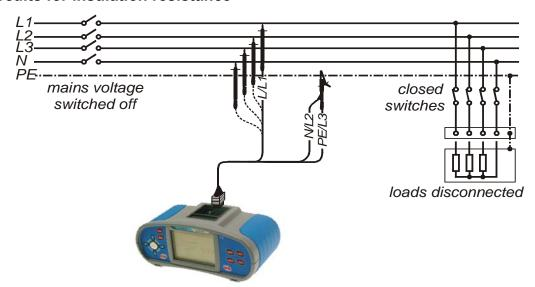
Figure 5.2: Connection of universal test cable for general insulation resistance measurement (TEST: L-PE)
