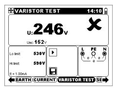
Figure 5.48: Example of varistor test result
