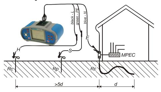
Figure 5.32: Resistance to earth measurement – PE grounding
